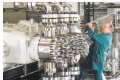
LEWA triplex process metering pumps
