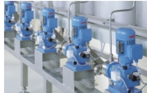
The LEWA ecodos pumps are working accurately in continuous operation ...
