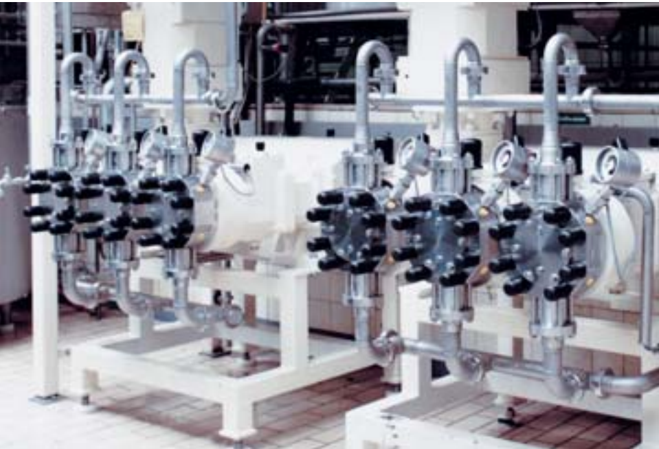
Example food production: gentle conveying of food-stuffs, 2 x G3 S, M500, 6 m 3 /h at 90 bar
